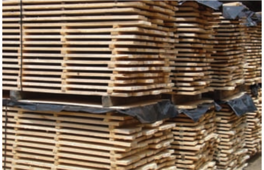
Once the wood is sawed, the lumber that will be made into flooring or paneling is air dried for six months, then kiln dried.
