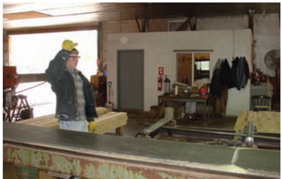
Eric Westerlund helps sort sawed lumber with hand signals that indicate what grade the product is.
