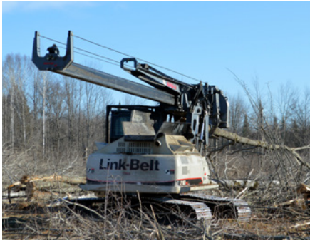
Trent Erickson operates a Link-Belt 210X stroke delimeter with a Pro Pac boom on Lyseng Logging's harvest west of Kelliher.
