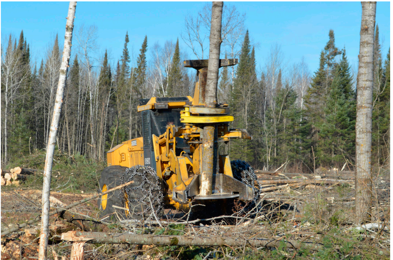
Steve Lyseng completes a clearcut with a John Deere 843H feller buncher.
