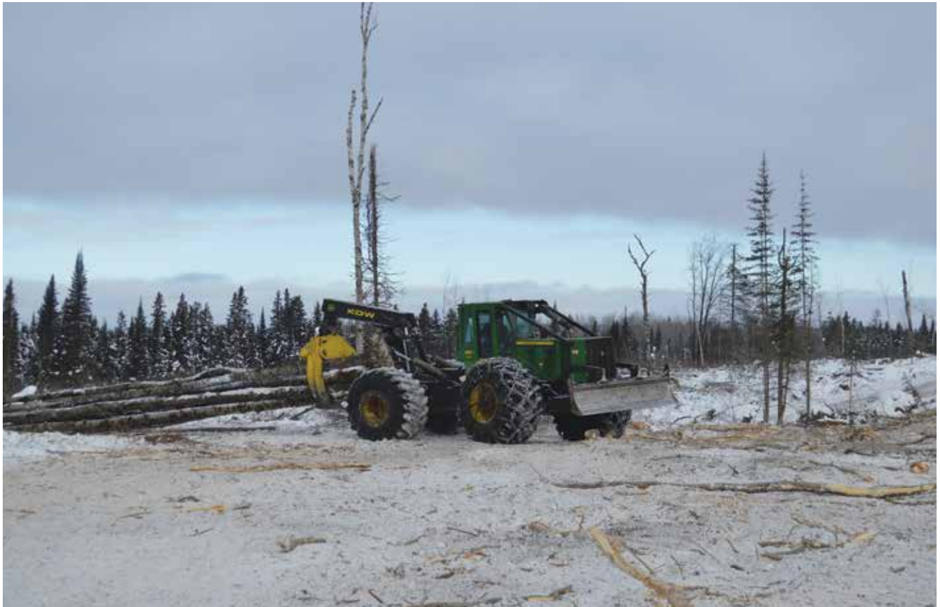
Bruce Stevens skids harvested timber with a John Deere 848H skidder. Krueger utilizes three skidders, including a 648H driven by Zach Gerard, and a John Deere 748H run by Jaxon Lind.
