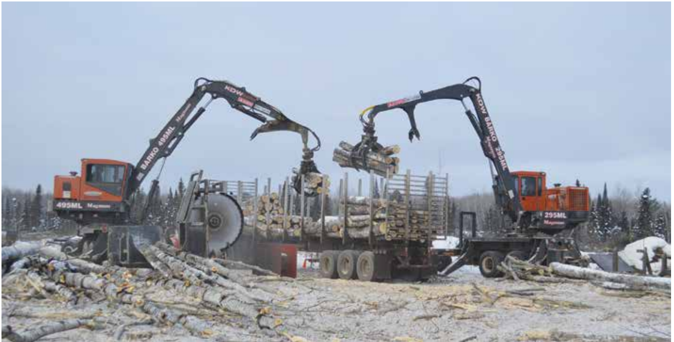
Krueger utilizes two Barko slasher/loaders to simultaneously load his trucks. Clint Krueger operates the 495ML Magnum, while Pete Klassen runs the 295ML.
