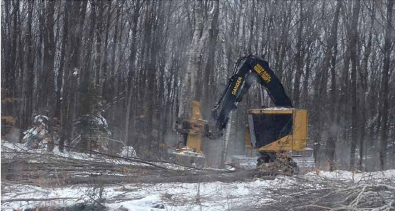
Justin Nukala runs Krueger's Tigercat 822 tracked feller buncher. Nukala often works ahead of the rest of the crew so that much of the timber has already been harvested when they arrive at the jobsite.
