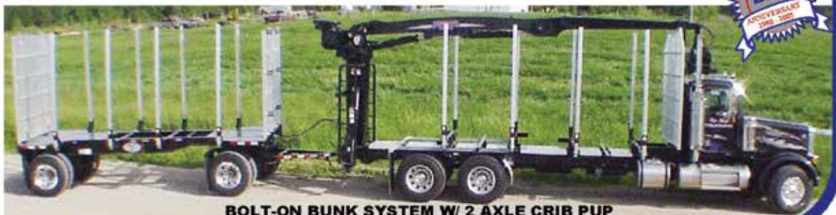
BOLT-ON BUNK SYSTEM W/ 2 AXLE CRIB PUP
