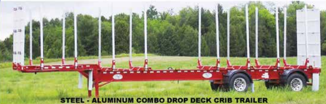
STEEL - ALUMINUM COMBO DROP DECK CRIB TRAILER
