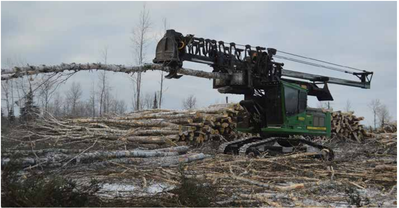
Allan Madson runs a John Deere 2154D stroke delimeter with a 2100C Lim-mit for KDW.
