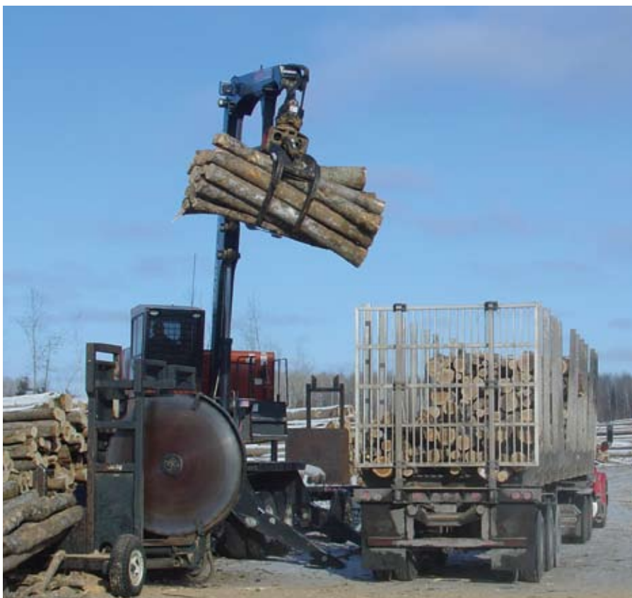
Kevin Leerssen (foreground) slashes and then loads 100-inch aspen on the landing with a 295 Barko loader and a HanFab slasher, while Joel Morrison (background) operates a 170 Serco loader, also with a HanFab slasher. Morrison and Leerssen also drive truck, as do Doug Siltman and Stephanie Stotler.
