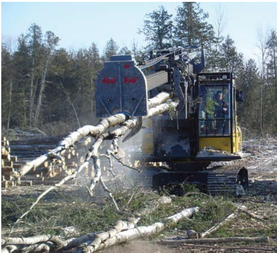
Glenn Dobbs delimits birch pulpwood, using a Propac on a Komatsu carrier. In addition, Dan Carriveau operates another Komatsu with a Propac on the same job.
