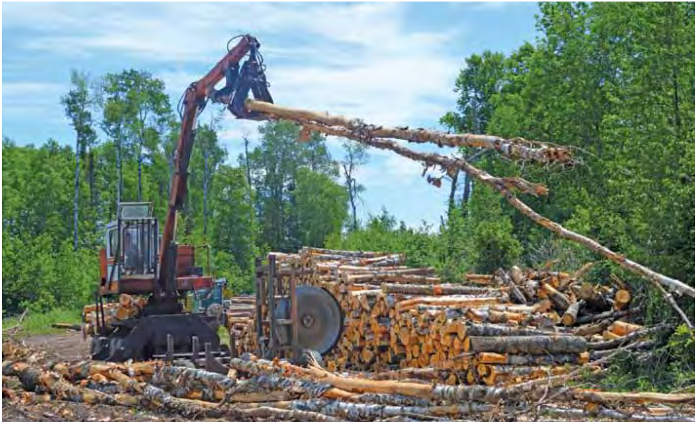
Kevin Kallinen processes harvested birch with a Serco 170-A loader with a 60-inch Siiro slasher.
