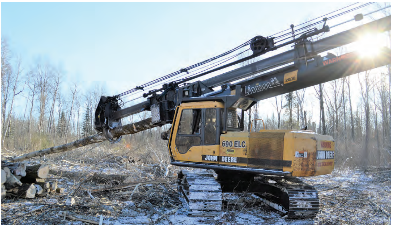
Walter Martins operates a John Deere 690 ELC delimeter with a Lim-mit 2000 boom for Rasmussen Logging.
