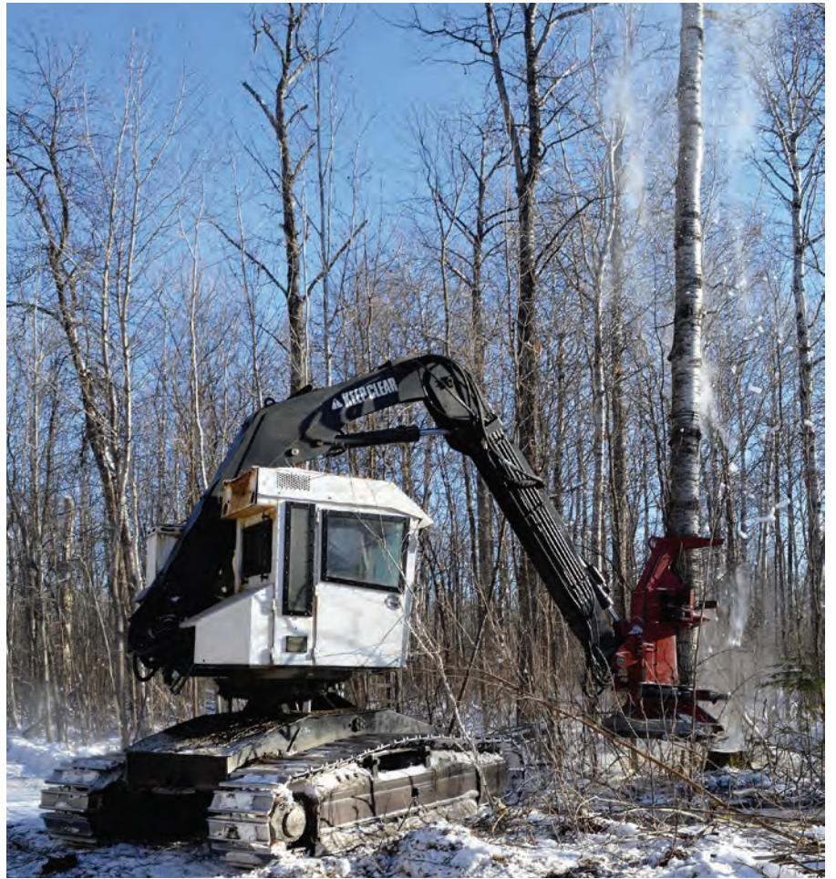
Jon Balaski harvests aspen with a Timbco 425 feller buncher. Rasmussen Logging also utilizes a Timbco 415 buncher.
