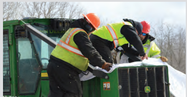
The crew at Enberg logging measures the company's skidder to make a pattern for a "Iron Nitey," to keep the machine warmer in extremely cold overnight temperatures.
