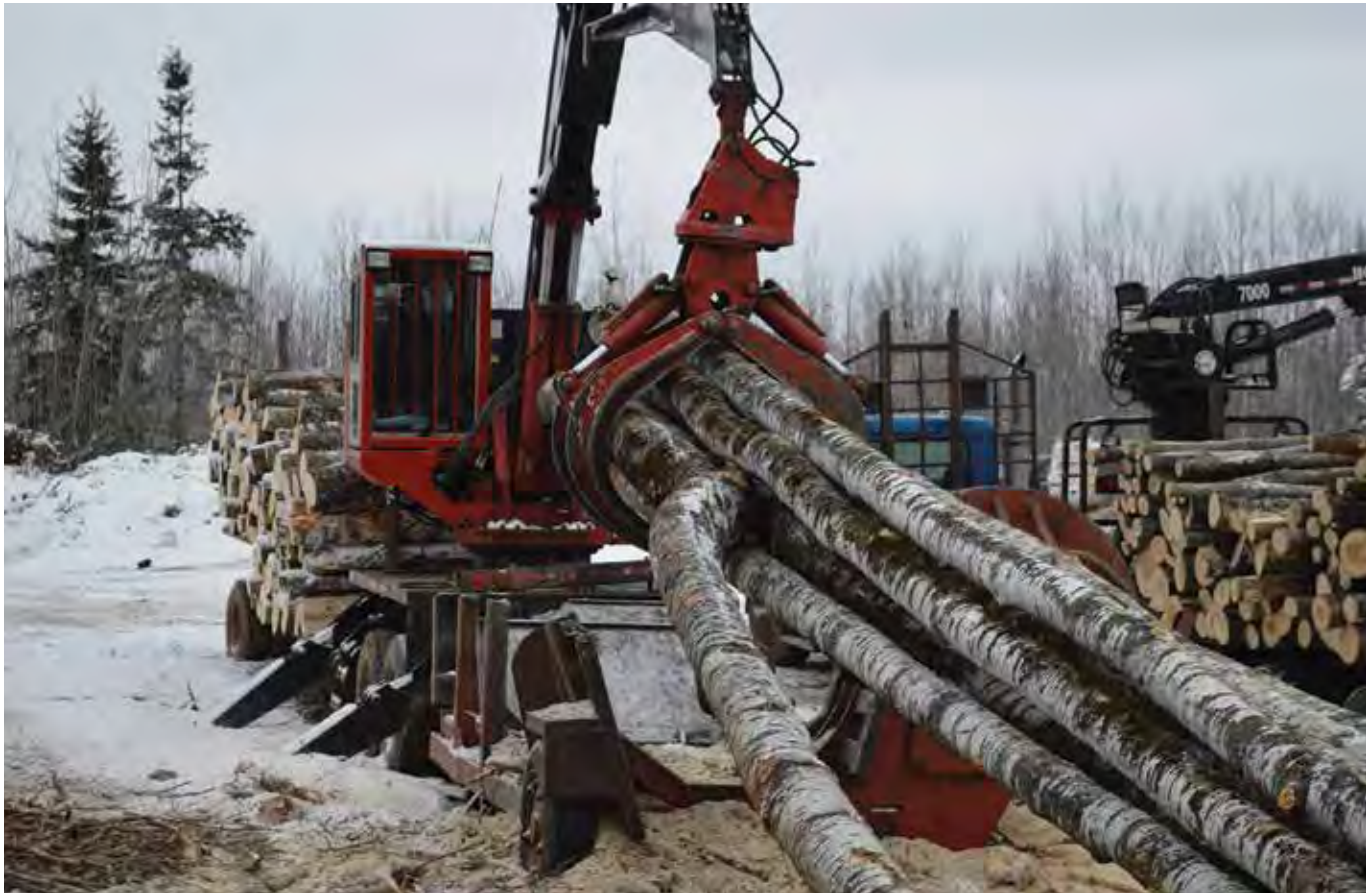
Lyle Jokinen places tree-length aspen into the Hood slasher to be cut into 100-inch lengths. Jokinen's father, Arnie, harvested this same site in the 1960s.
