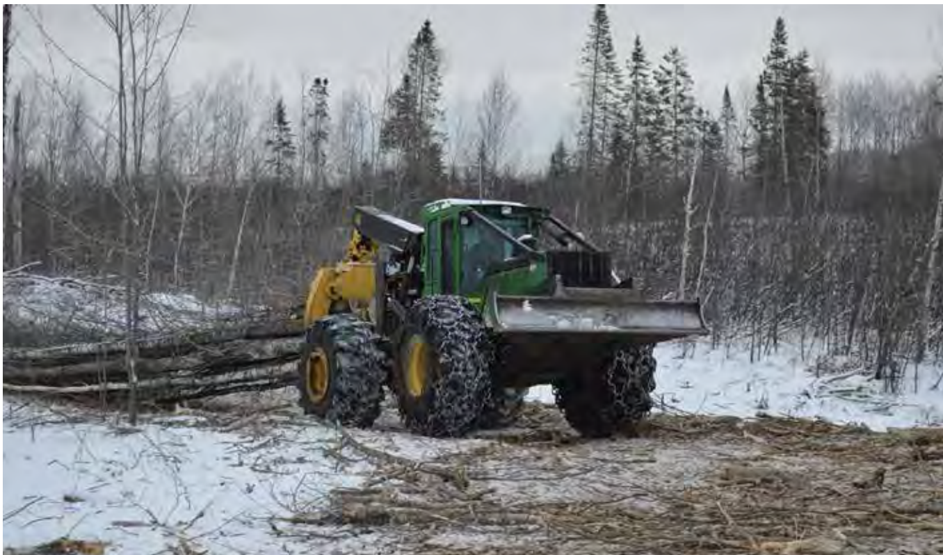
Ryan Olesiak, Dave's son-in-law, drags harvested aspen to the landing with a John Deere 748G-III skidder. Berthiaume Logging also utilizes a Tigercat 620C skidder driven by Dave's nephew, Andrew Berthiaume.
