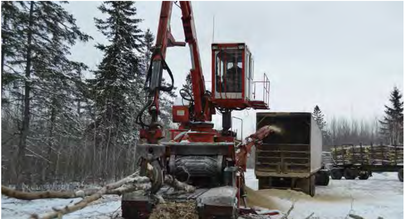
Derek Jokinen loads aspen limbs and tops into a Morbark chipper with a Hood loader. The chips are being blown into a chip van for transport to Sappi in Cloquet.
