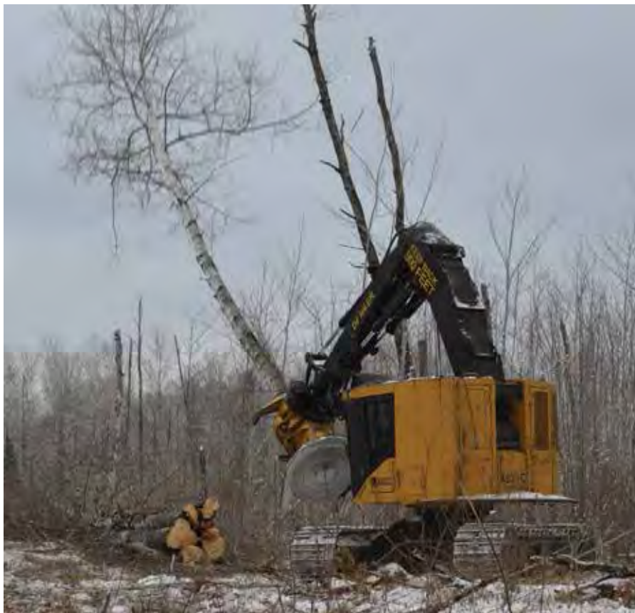
After severing an aspen tree with the Tigercat X822C feller buncher, Bob Berthiaume lays the tree down for efficient skidding to the landing.
