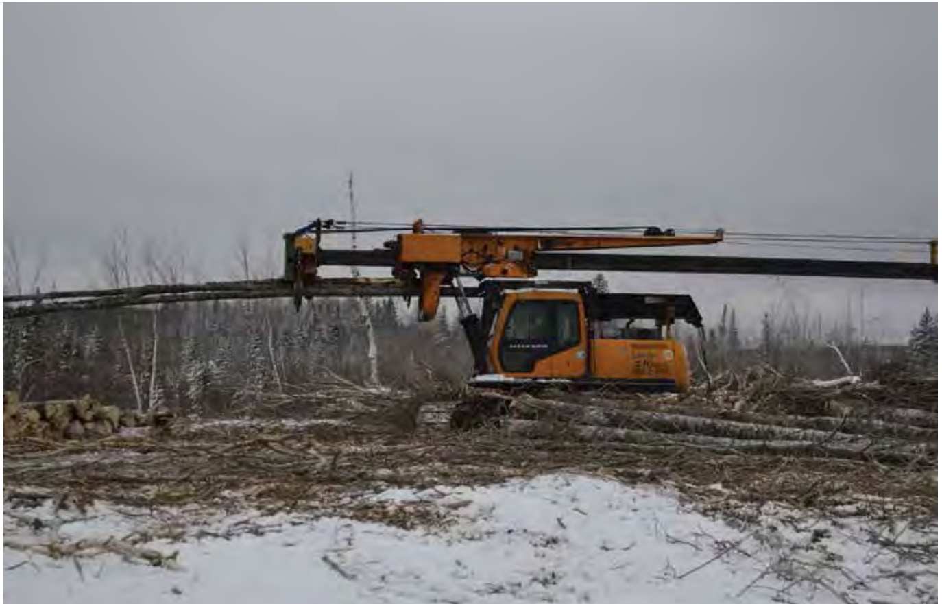
Derek Jokinen operates Berthiaume's Hyundai delimeter with a Pro Pak boom.
