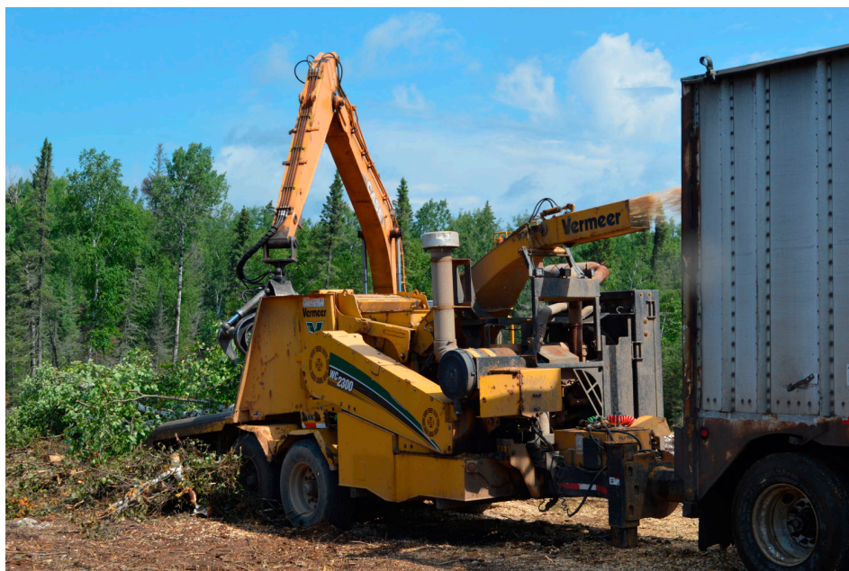
Tops and limbs are fed into a Vermeer WC 2300 chipper to manufacture biomass.
