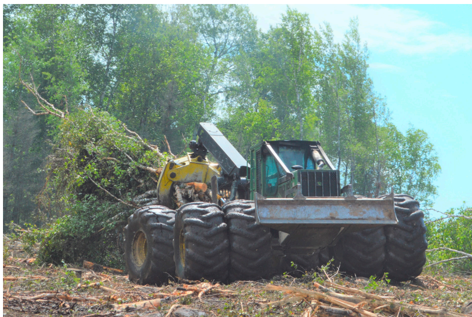
Waste Wood utilizes "duals" on one of its skidders in the summer time to better operate on softer ground.
