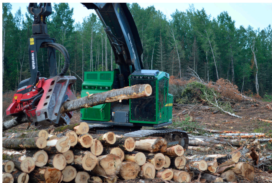
Garon Campbell operates the recently purchased John Deere 803MH processor, which replaces a stroke delimber and slasher on Waste Wood's landing.
