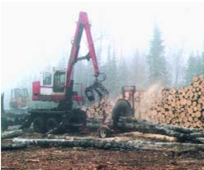
Tony cuts the aspen into 100-inch lengths with the Serco loader and Siiro slasher.
