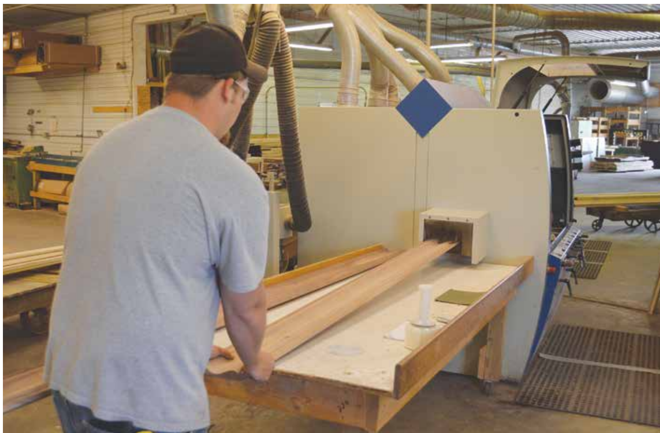
Trevor Lang operates the machine that makes crown molding. Each piece is cut to order at Root River's facility adjacent to the showroom on the northern edge of Preston.
